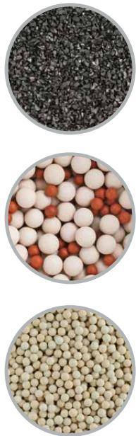
In contrast to conventional activated carbon blocks, the flow rate of MAUNAWAI® filters is significantly reduced. This supports the increased bonding capacity of the granulate used. The **high-tech activated carbon made from coconut shells** removes contaminants such as chlorine, pesticides, heavy metals, and many other impurities. In the threshold range of substances that are difficult to bind, such as copper, zinc, and antibiotics, MAUNAWAI® filters prove to be advantageous.
