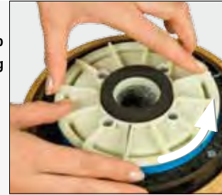
Figure 6 Unscrew the top stone by turning it counterclockwise.
