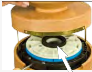
Figure 4 Make sure the foam rubber gasket is properly seated (arrow). Return the funnel to its previous position and secure it with the brass screws.
