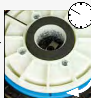
Figure 8 When screwing the grindstone back into place, make sure that it does not tilt.
