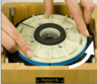
Figure 6 Remove the top grindstone by turning it counter-clockwise
